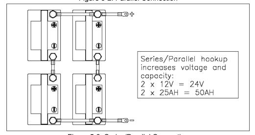
Figure 5-3. Series/Parallel Connection
