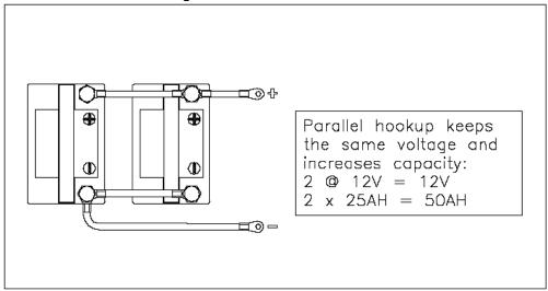
Figure 5-2. Parallel Connection
