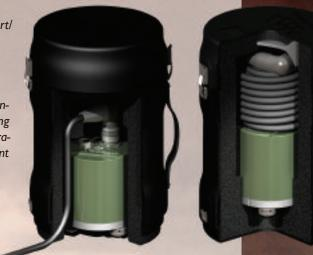
Trillium Compact combines the superior performance of a broadband seismometer with the installation convenience of a rugged geophone. The instrument incorporates a symmetric triaxial force feedback sensor design with a response flat to velocity from 120 seconds to 100 Hz.
