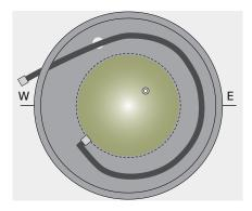
8. Orient the connector groove in the cover to the connector and place the cover over the seismometer.
