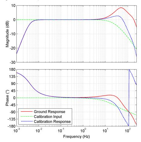
Table 10-1 provides the ground motion response nominal parameters. The ground motion response has -3 dB corners at 244.2 s and 223 Hz. The ground motion sensitivity at  $f_0$  specified in Table 10-1 assumes an infinite input impedance at the digitizer. For digitizers with low input impedance, it will become necessary to account for the fact that source impedance of the differential outputs is 300  $\Omega$ ,  $\pm 1$  percent (150  $\Omega$  for each output).
