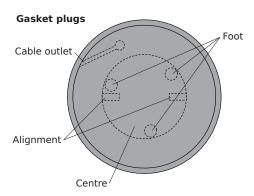
A standard installation retains the original position of the cable outlet and leads the cable around the base of the gasket, enclosing approximately 1 m of cable in the cover. Enclosing the cable in the cover helps attenuate temperature variations conducted by the cable.
