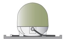
6. Pull the cable end through the cable outlet.
