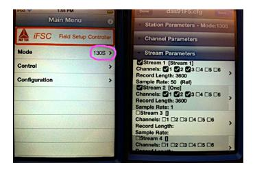
Mixed 50sps stream configuration of a PASSCAL RT-130 with the 3.4.3 FW using this method (using 130S Mode) is possible. Note that this sample rate is not compatible with the new real time data monitor function (see 3.4.0-7 above).
