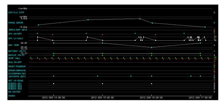
209:15:40:00 EXTERNAL CLOCK POWER IS TURNED ON 209:15:40:05 EXTERNAL CLOCK IS UNLOCKED 209:15:44:42 EXTERNAL CLOCK IS LOCKED 209:15:45:34 INTERNAL CLOCK PHASE ERROR OF 4 USECONDS 209:15:46:49 EXTERNAL CLOCK IS UNLOCKED
