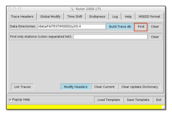
Build Trace db loads your \*.m files. Once you select Build Trace db a window pops up telling you that the trace db is being built. This could take a few minutes depending on how many files you are loading.
