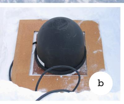
Figure 2: Seismic vault (a) and Trillium 240 installed on phenolic block (b).
