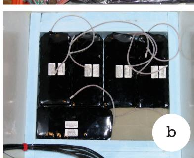
Figure 1: Station enclosure (a) and lithium thionyl chloride battery pack (b).
