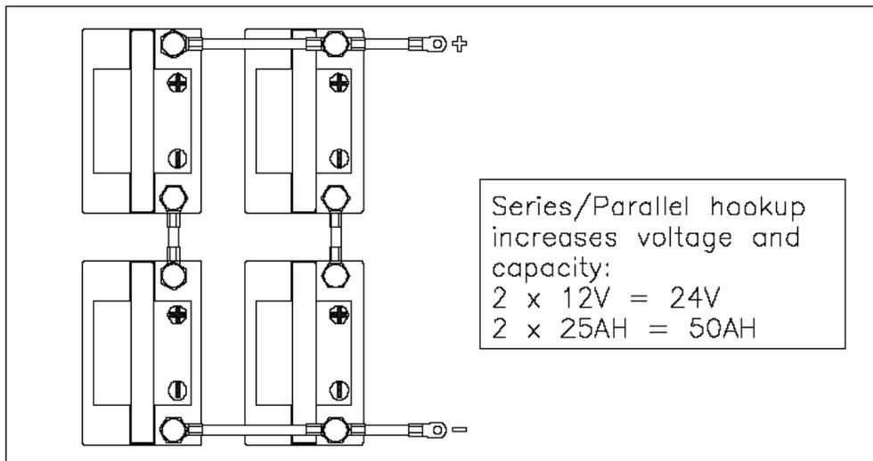
Figure 5-3. Series/Parallel Connection
