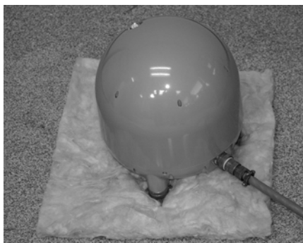
Figure 3-1 Fibreglass batt insulation under the Trillium 240
