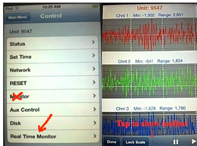
NOTE: This function only works with Group 2 sampling rates (see 3.4.3-5 below for list of sample rates in each group), except it does not work with the 50 sps rate newly added to Group 2.
