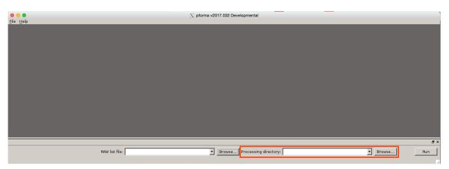
Increase timeout: File > Set Timeout. For Texans, the default timeout (2000 seconds) should be sufficient but when processing data from RT130s, increase the timeout by factor of 10.
