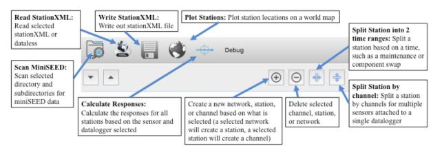
Buttons in the main Nexus GUI. The Split Station buttons can be used to create new time epochs (for a service run that involved a sensor or datalogger swap) or separate out channels for a station with multiple sensors.
