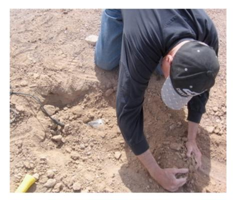
Tamp down the dirt around the sensor as you fill in the hole.
