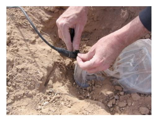
Tape around the cable just beyond the connection into the sensor and seal all open edges of the bag.
