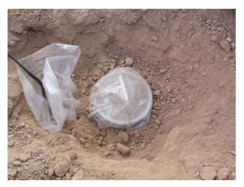
Pack dirt or sand along the outside of the bag all the way up the sensor and gently compact to keep the sensor level.
