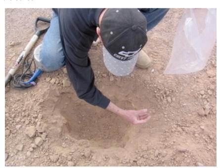
**Tip 4** – For a short-term experiment (less than 2 months, and not very wet environment) direct burial of the L-22 is okay. For a long-term experiment (more than 2 months) or in a very wet environment the sensor should be protected from flooding by burying it in a plastic bag. Place the instrument in the bag with the top of the bag open in your pit.
