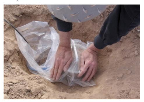
Level the instrument, making sure that you can see the bubble level, and pull the bag up.
