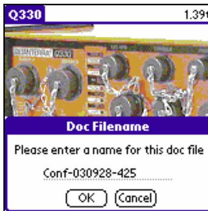
3. When the Q330 control program has finished quit it (by tapping the Applications button -- the "house" icon to the left of the Grafitti area). Check that the Launcher category setting in the upper right-hand corner of the display is set to "All" and find the icon for the application FileZ. Start the FileZ program by tapping on its icon.
