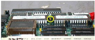
Flip the card over and short out the pins of the capacitor for a couple seconds. C12 may not always be labeled on the back of the PC board.
