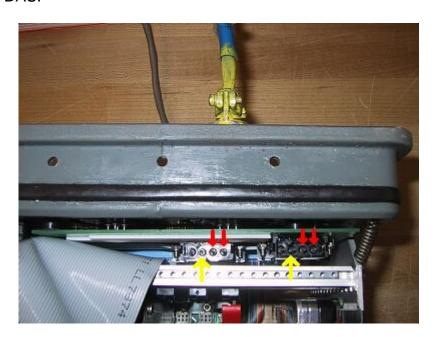
If everything above is OK, disconnect the 12v power source from the front of the DAS, and reconnect the internal cable to the connector on the back of the front panel.
