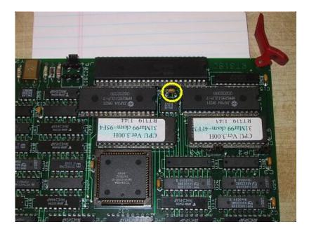
On some CPU cards a PC board as in the picture below may cover C12. C12 will be hiding beneath it.
