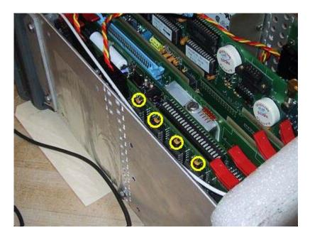
Check the voltage across any one of them. There should be 5v. If there is not then it means that the power supply card is broken and will need to be replaced.
