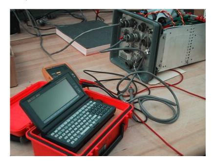
Assuming the DAS did not "come to life" when it was connected to power, locate the four capacitors on the power card.
