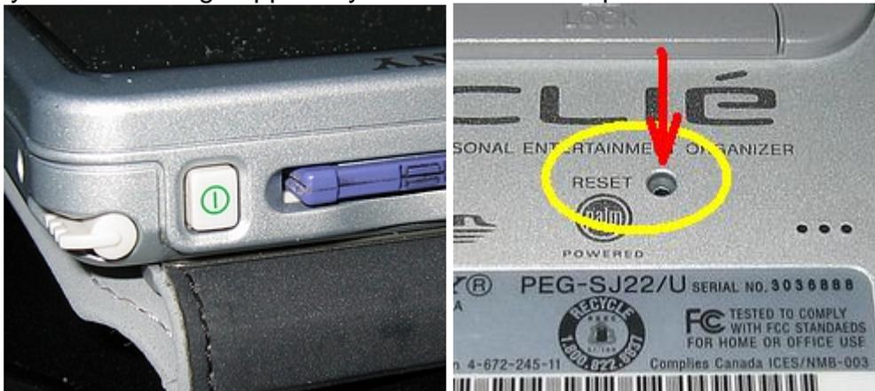
2. When the power button is released the question "Erase all data?" will appear. Push the rocker button (the center button of the 5 hardware buttons below the display) up to erase everything. The Palm Powered logo will return and the unit will reboot.
