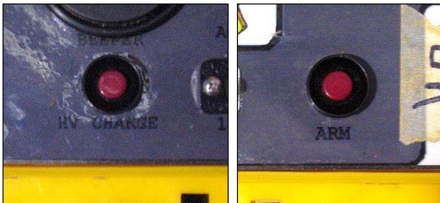
10. **KABOOM.** At the correct time (on the minute in this example) the trigger and detonation pulses will be generated. The HV CHARGE and ARM buttons may be released. If you do not want a trigger pulse to be generated the next minute then press the CANCEL button to leave the countdown display.
