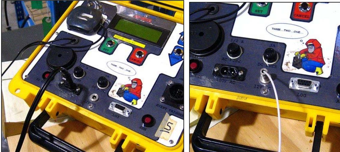
2. **Set up the GPS antenna.** When you are ready to operate the shot box remove the GPS antenna from the Velcro on the shot box and place it where it will have an unobstructed view of the sky. If the whole shot box has an unobstructed view of the sky then the GPS antenna may be left attached to front of the shot box. There is about two meters of cable connected to the GPS antenna.
