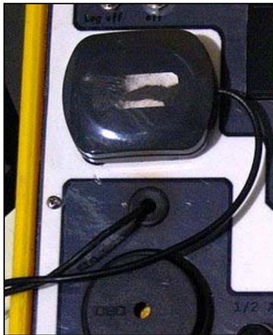
3. **Turn on the power** using the power switch in the upper left-hand corner of the front of the box.
