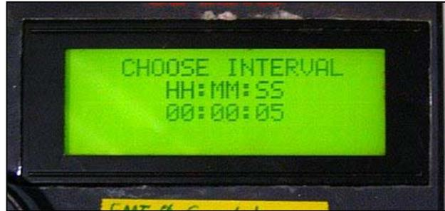
Use the UP and DOWN buttons to set the interval to what you want to use. A one minute interval is what would be consider "normal" (the picture below). This means that a trigger pulse will be generated every minute ON the minute. When you start the countdown you will have one minute or less before the trigger pulse gets generated. Once you have the interval you want to use selected press the SET button to set it and leave the display.
