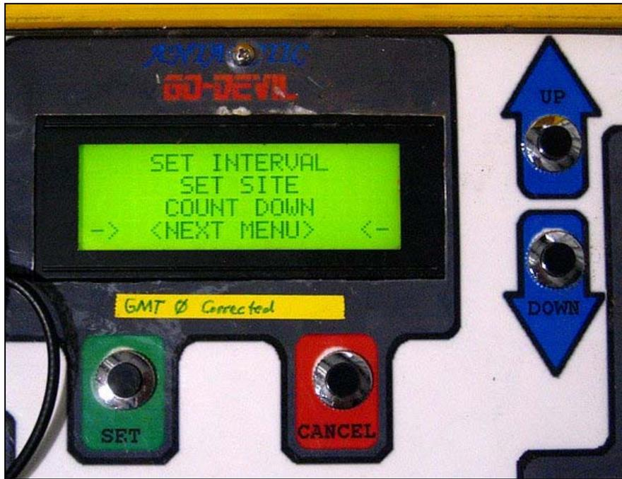
6. **Setting the interval.** The shot box will generate a trigger pulse at set time intervals. This interval can be set through the SET INTERVAL menu item and it **SHOULD BE DONE EVERY TIME YOU TURN THE SHOT BOX POWER ON.** From the main display with the time and position press the SET button. This will take you to the menu in the picture below.
