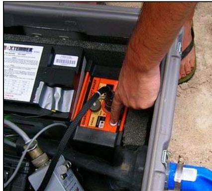
**6. Disconnect the baler.** If the baler is to be swapped with a clean one then disconnect the QNET cable from it and connect the new baler in its place. Use the Clie control program (described above), or press and release the ATTN button on the new baler and check to see that it boots up and receives some data from the Q330 to verify that it is connected properly.
