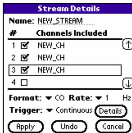
10. A format of CO (compressed) is OK. A Trigger setting of Continuous is also OK. Tap on the Details button and set the Record Length to 3600 on the Continuous Trigger dialog box. A future start time can also be set on this dialog box if needed, but it is usually left alone. Tap OK to return to the Stream Details display. Change the Rate setting by tapping on the down arrow to the right of the Rate label and selecting 50 (samples per second). Tap the Apply button when finished.
